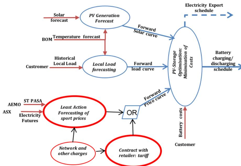
**Figure 1. Research Method: forward solar, load and price curves are combined to derive battery charging and electricity export schedules minimising overall cost of consumed electricity.**
