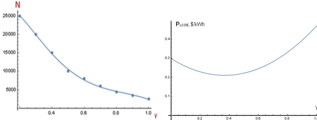
**Figure 3. Number of cycles as a function of DOD (left) and Dynamic LCOE as a function of DOD (right)**
