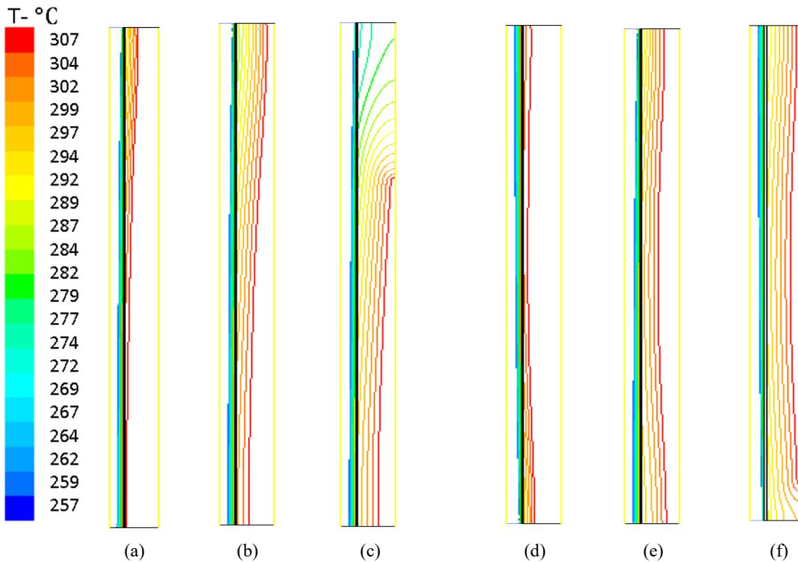
**Figure 3. Isotherm evolution during solidification process, steady boundary:**
