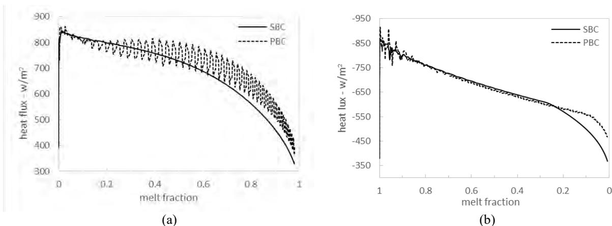
FIGURE 4. Temporal evolution of heat flux a) melting, b) solidification
