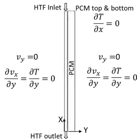
**Figure 1: Schematic of the model, including boundary conditions**
