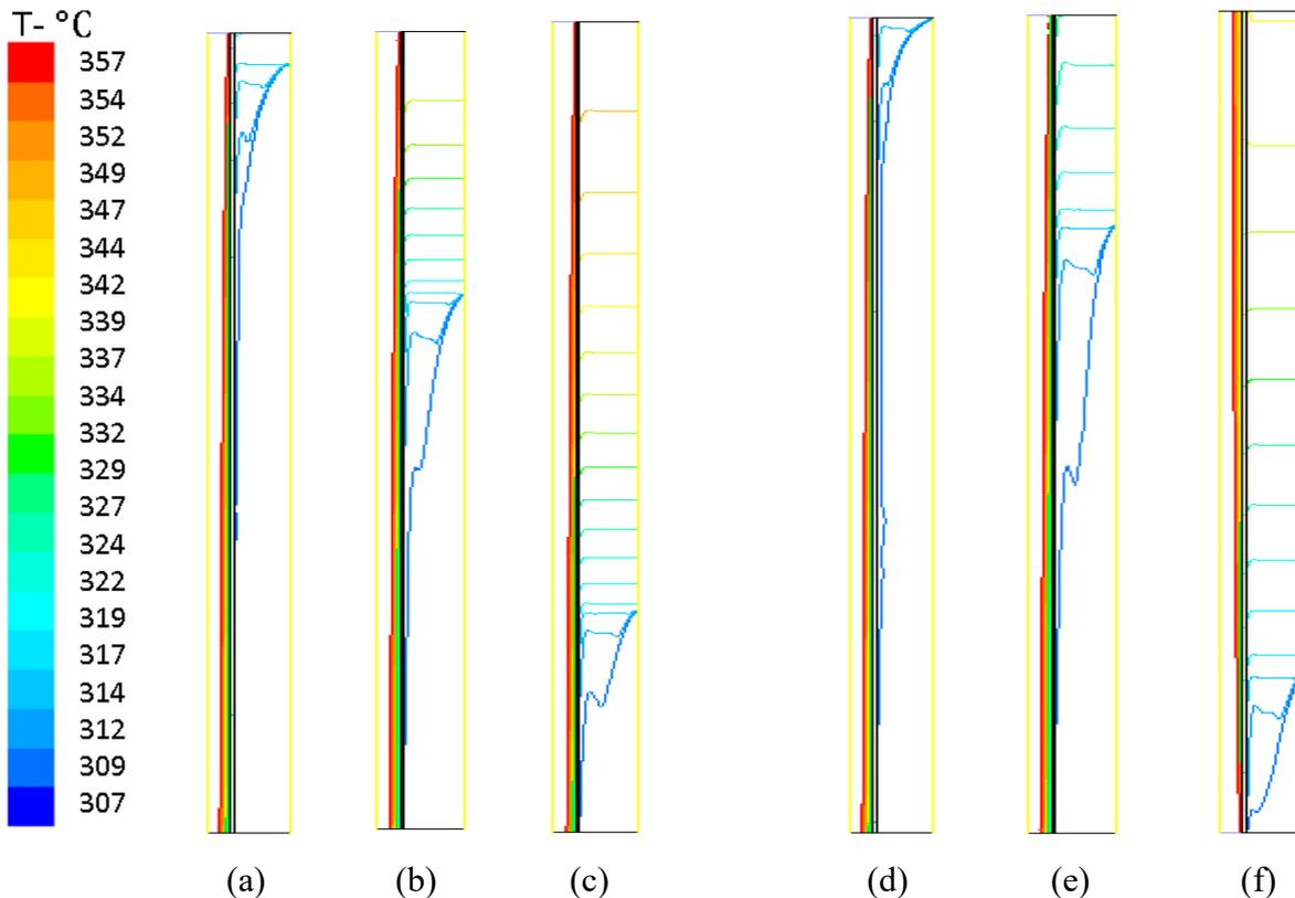
**Figure 2. Isotherms evolution during melting processes, steady boundary:**
