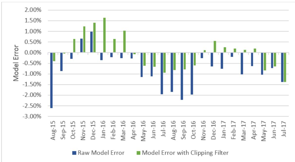
**Figure 8 – Reduction in model error when the clipping filter is applied**
