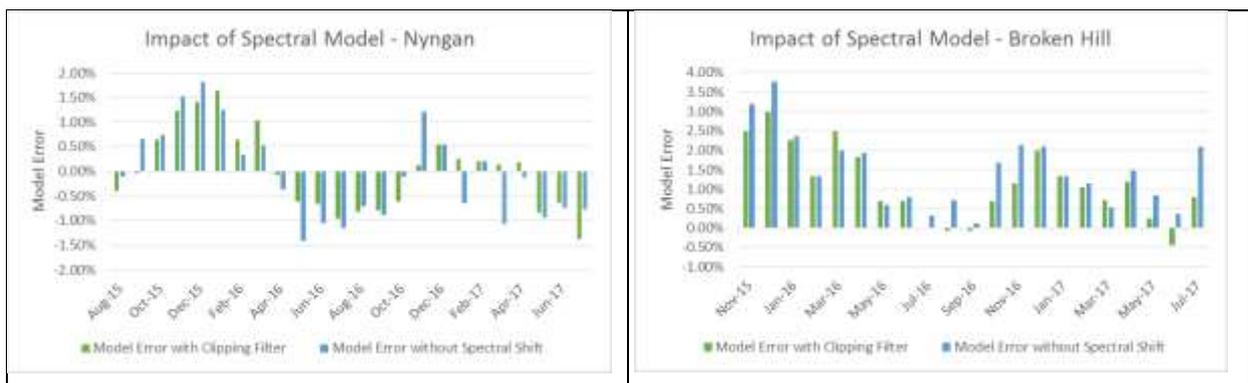
Figure 9 – Reduction in model error from inclusion of spectral model
