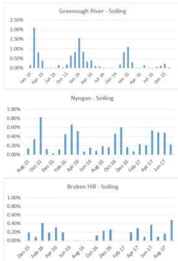
Figure 2 - Actual measured soiling at Greenough River, Nyngan and Broken Hill Solar Plants
