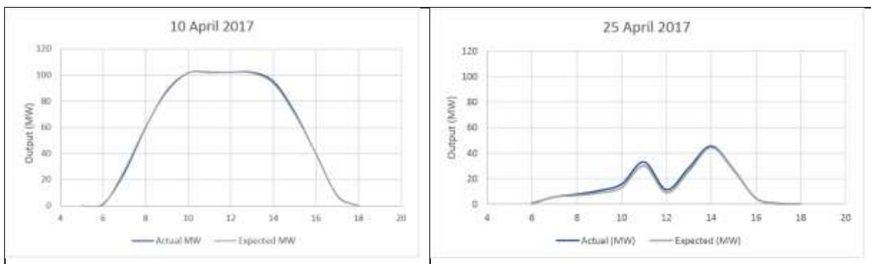
Figure 6 – Generation profile for typical sunny and cloudy days at Nyngan
