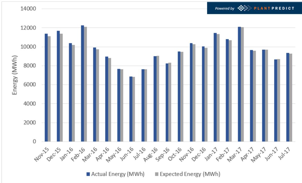
**Figure 4 - Broken Hill Solar Plant actual vs. expected performance modelled in PlantPredict (BHSP 2017)**
