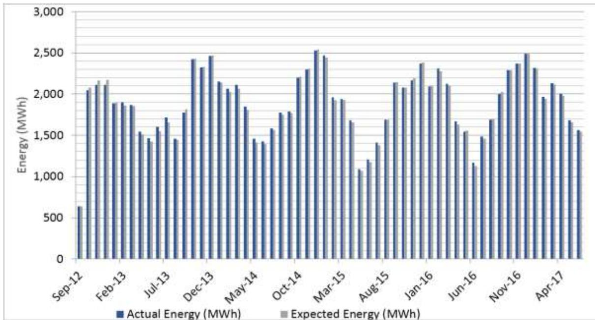
Figure 5 - Greenough River Solar Farm actual vs expected site performance using irradiance-scaling methodology and including lost energy adjustment (GRSF 2017)
