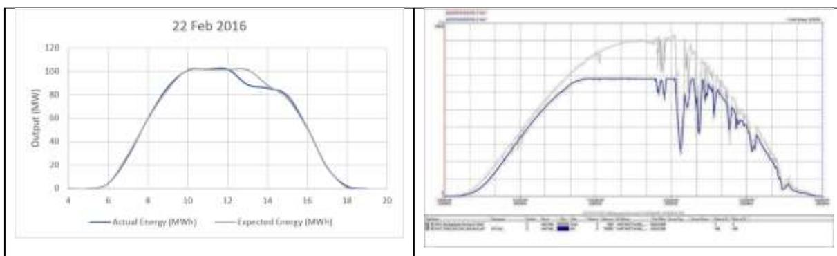
**Figure 7 – Generation profile (left) and 1-second generation vs irradiance (right) for a partly clear, partly cloudy day at Nyngan**
