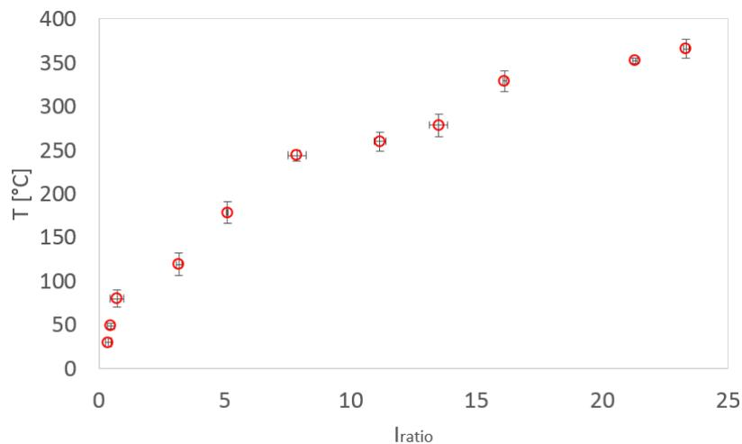
Fig. 2: Calibration curve relating phosphorescent emission of ZnO:Zn to temperature, where intensity ratio was calculated by superpositioning and dividing images taken with filters at  $440 \pm 20\text{nm}$  and  $392 \pm 9\text{nm}$ .
