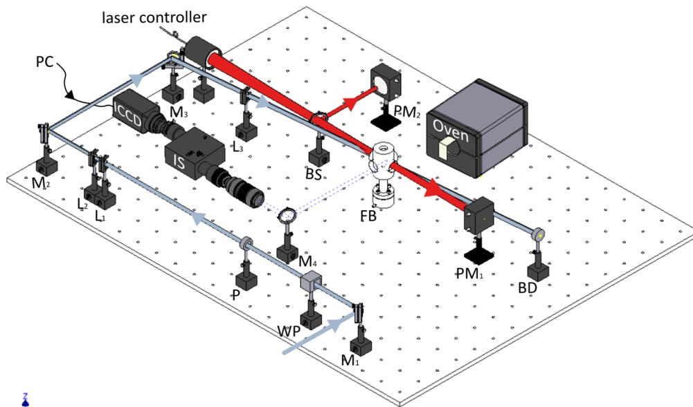
Fig. 1. Optical arrangement. Note that the temperature-controllable oven replaces the fluidized bed during calibration. Purple line: 355nm Nd:YAG laser beam path; Red line: 910nm Solid-State Solar Thermal Simulator (SSSTS) beam path; Blue dashed line: optical collection path of phosphorescence emission. BD: Beam Dump; BS: Beam Splitter; FOC: Fibre-optic Cable; ImL: Imaging Lens; L: Lens; M: Mirror; P: Polariser; PM: Power Meter; sp: spacer; WP: Waveplate.
