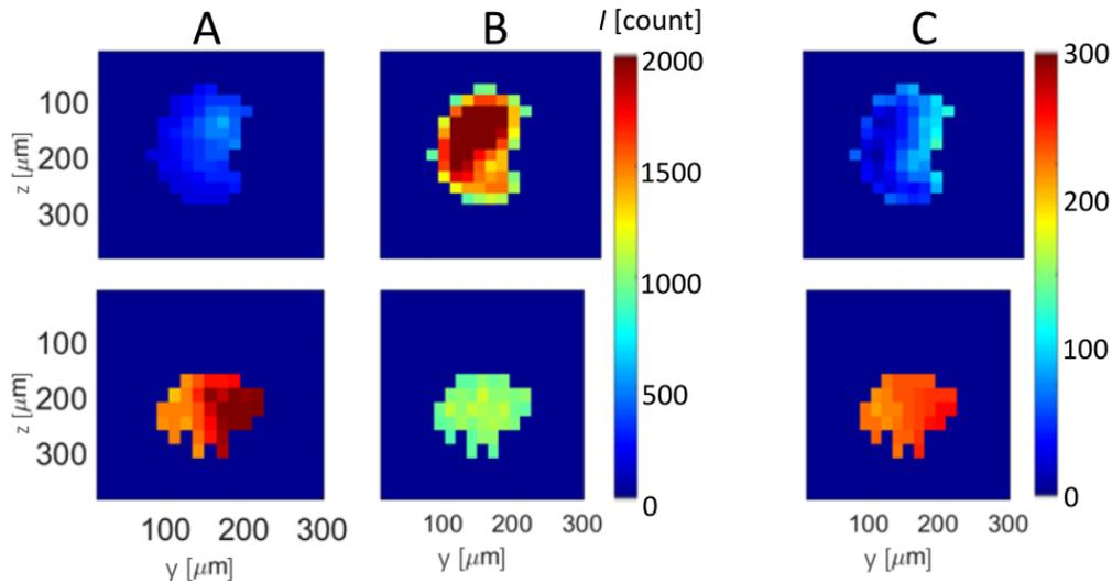
Fig. 3: Typical examples of image trios of particle agglomerates, comprising raw image pairs  $420 \pm 20\text{nm}$  (column A) and at  $392 \pm 9\text{nm}$  (column B), together with the resulting temperature,  $T_p$  (column C), recorded for five values of radiative heat flux,  $\Phi$ : (1)  $0 \text{ MW/m}^2$  and (2)  $12.4 \text{ MW/m}^2$ .
