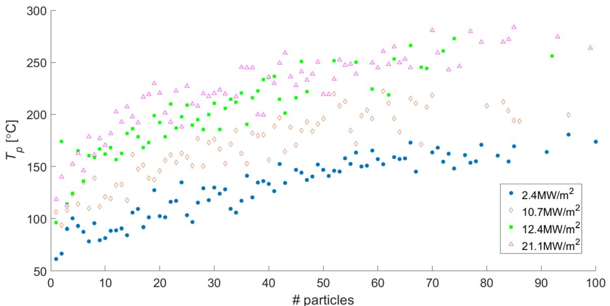
Fig. 6: Dependence of particle temperature on the number of particles per image at  $\Phi = 2.4 \text{ MW/m}^2$ ,  $10.7 \text{ MW/m}^2$ ,  $12.4 \text{ MW/m}^2$  and  $21.1 \text{ MW/m}^2$ .
