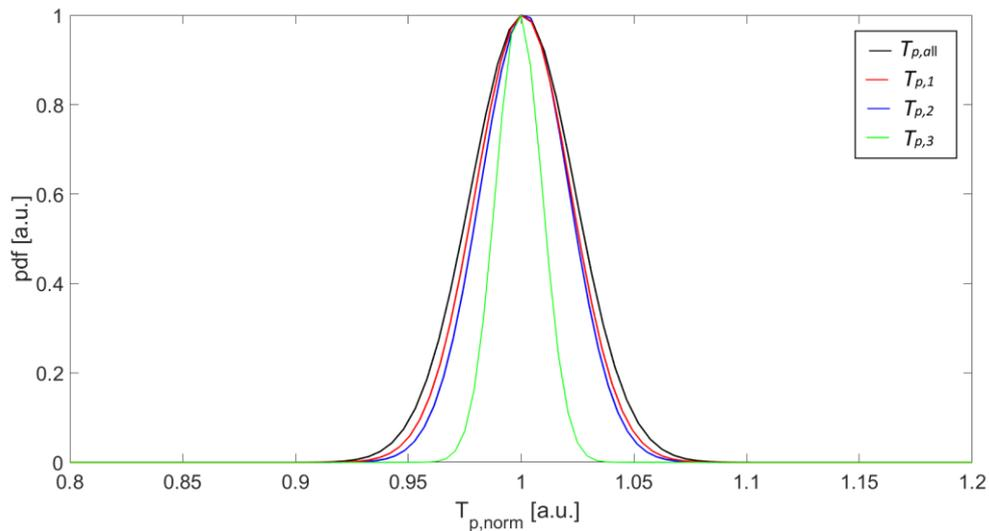
Fig. 4: Probability distribution comparison of particle temperatures,  $T_p$ , where  $T_{p,all}$  was calculated based on all  $T_p$  over 650 captured images, while  $T_{p,1}$ ,  $T_{p,2}$ ,  $T_{p,3}$  are the temperatures of single particles.
