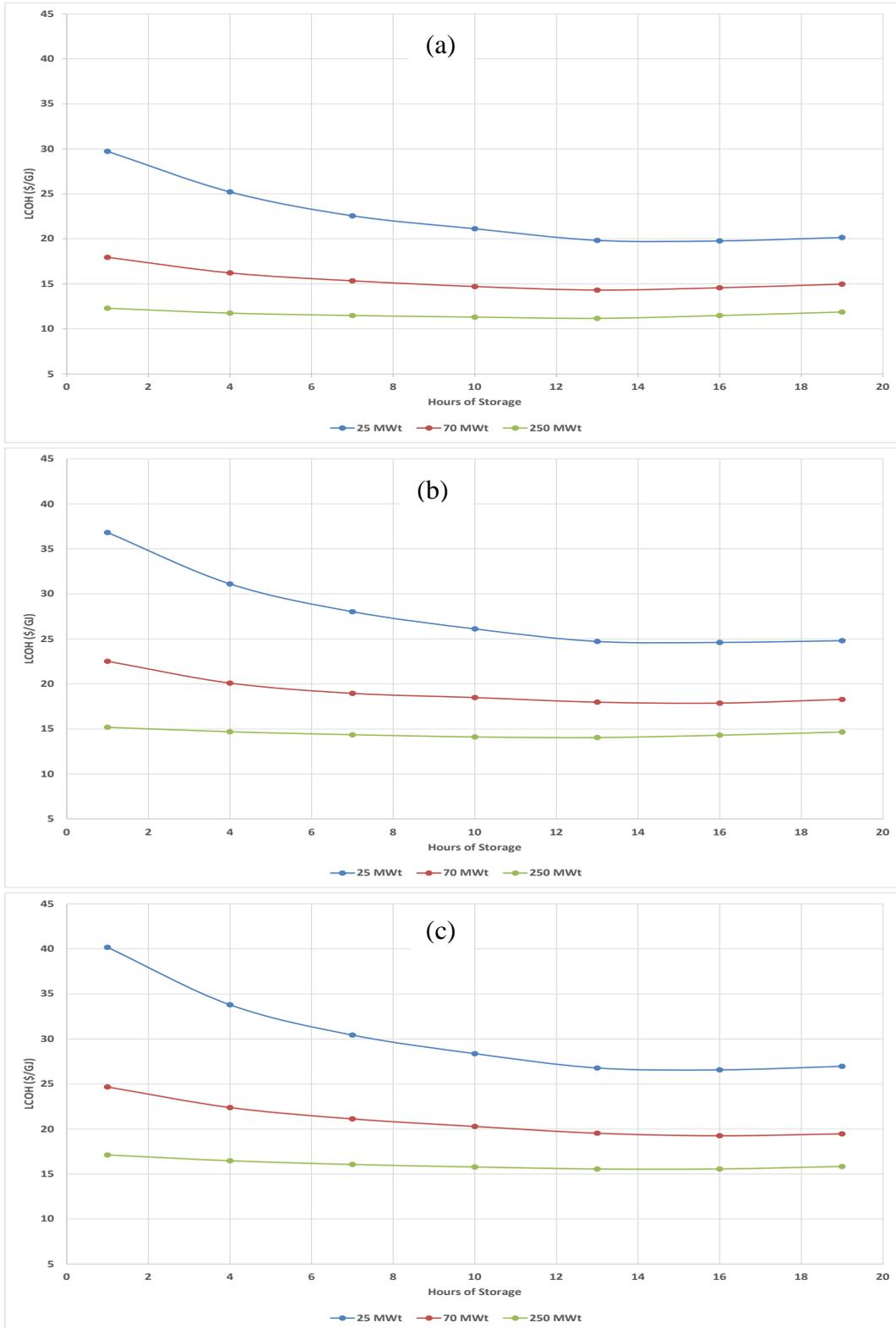
Figure 3. LCOH versus the thermal storage capacity: a) Learmonth; b) Kalgoorlie; c) Rockhampton
