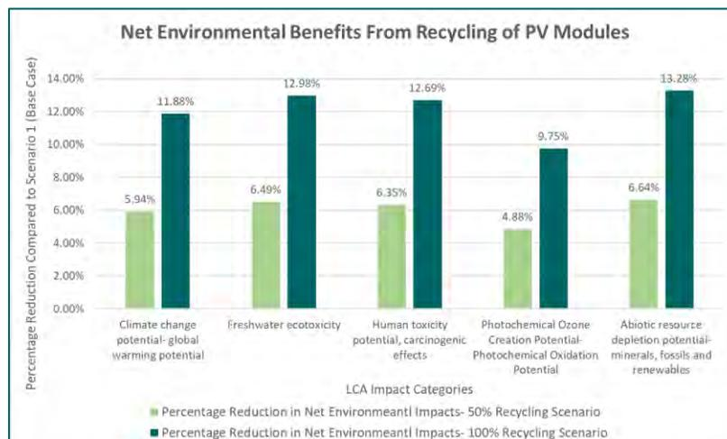
**Figure 2. Net environmental benefits from the recycling of PV modules**
