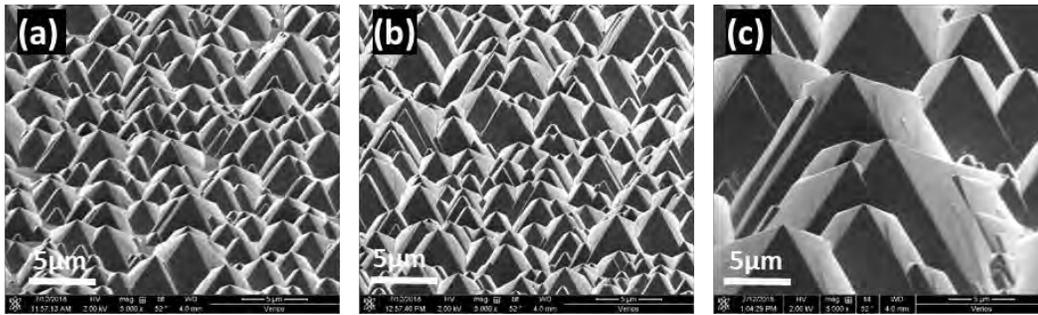
Figure 2 Compare the morphology of textured Si surfaces with different texturing solution. (a) TMAH-monoTEX, (b) KOH-monoTEX, (c) TMAH-IPA
