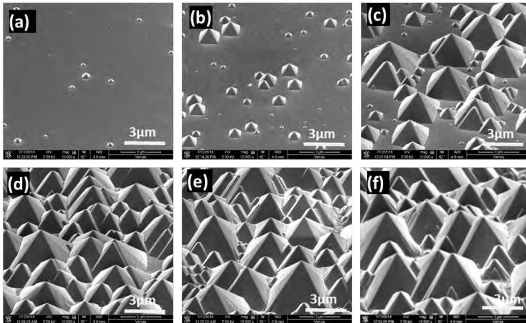
**Figure 1** Emerging of pyramids during a TMAH-monoTEX texturing process. (a) 2min, (b) 4min, (c) 8min, (d) 12min, (e) 20min, (f) 30min. A magnification factor of 10000X was used for all the images.
