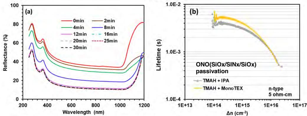
Figure 3 (a) Reflectance evolution with TMAH-monoTEX texturing time; (2) Lifetime curves for TMAH-IPA and TMAH-mono textured silicon samples
