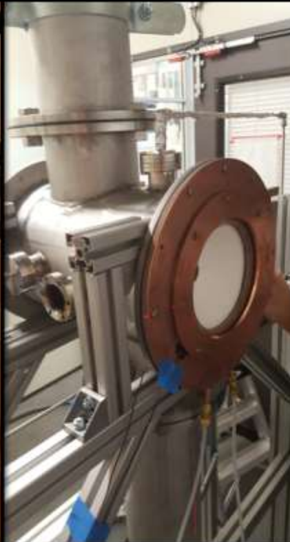
Water-cooled copper diaphragm with quartz window
