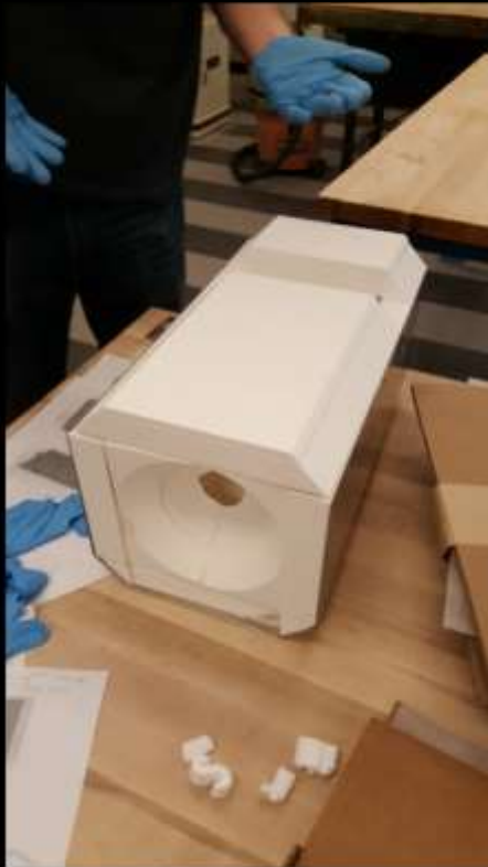
Fully fabricated SR3 cavity made of alumina
