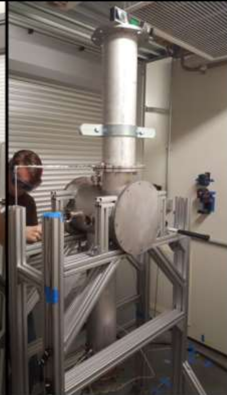
SR3 mounted in front of the HFSS with hoppers
