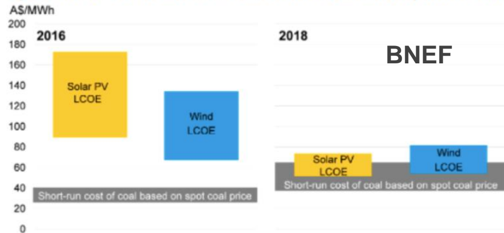
Figure 2: Short-run cost of coal versus levelized cost of electricity of wind and solar
