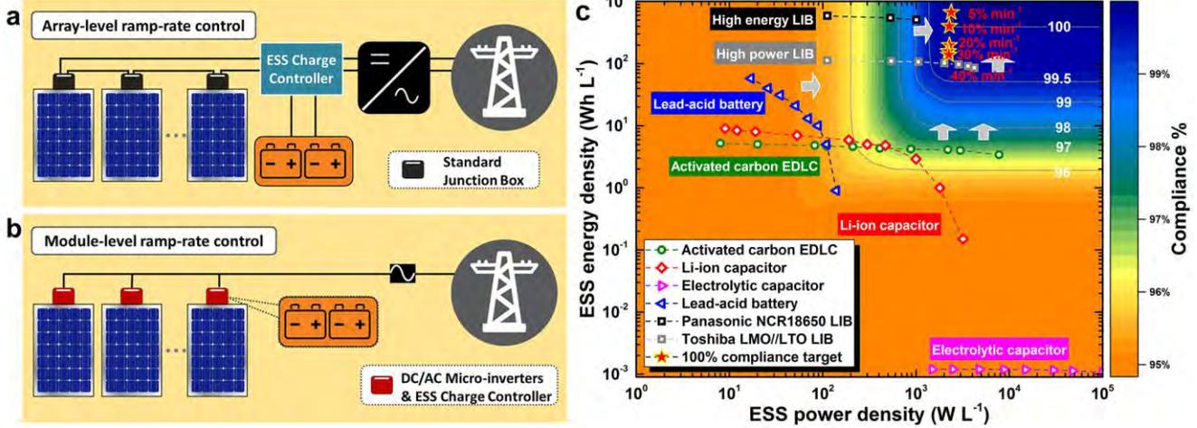
**Figure 1.** Configuration of a PV system with an ESS for ramp-rate control at the a) array level and b) module level. c) Achieved levels of compliance for a ramp-rate limit of 10% min<sup>-1</sup> when the ESS volume is restricted to 0.1 L.
