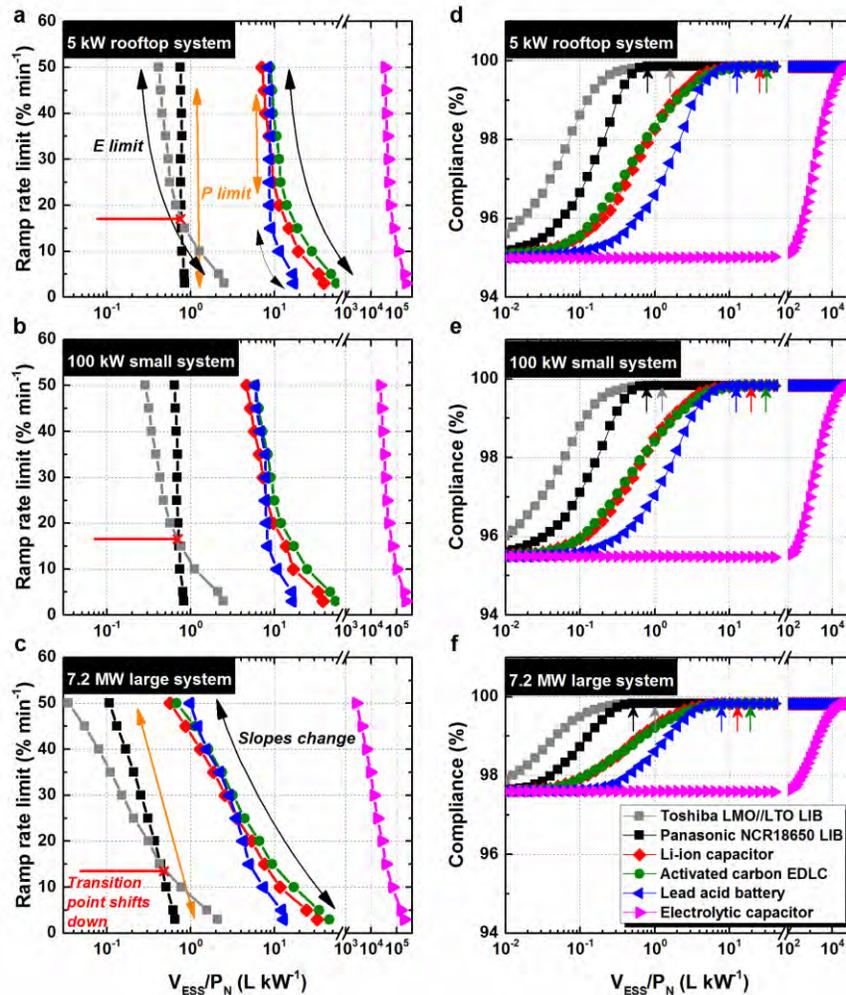
**Figure 2.** Calculated ESS  $V_{ESS}/P_N$  requirements for different allowable ramp-rate limits for three PV system sizes.
