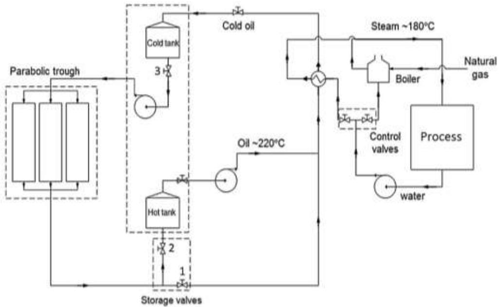
**Figure 1. A schematic diagram of the proposed process, hybridising a mid-temperature process with concentrated solar thermal energy. Storage tanks are employed to store hot and cold oil as the working heat transfer fluid.**
