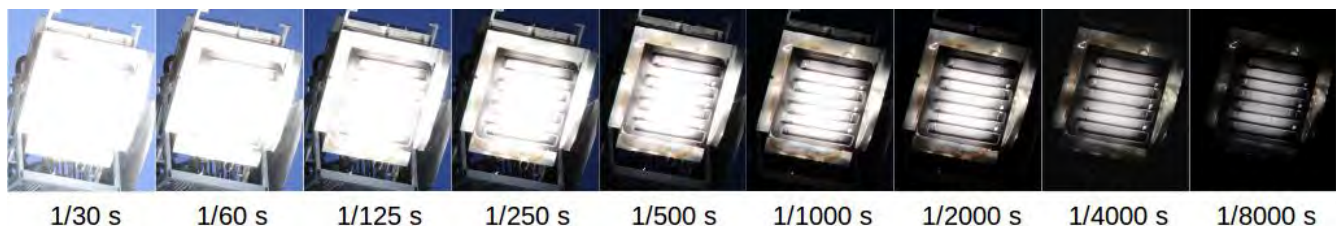
Figure 1. Demonstration of images with different exposures (shutter speeds) of the bladed receiver under high flux irradiation.
