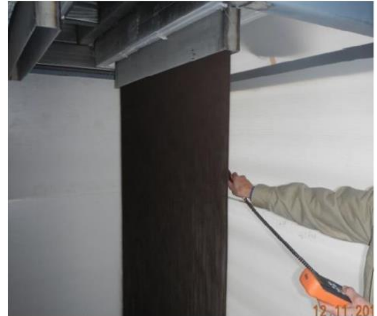
Free-falling particle curtain
