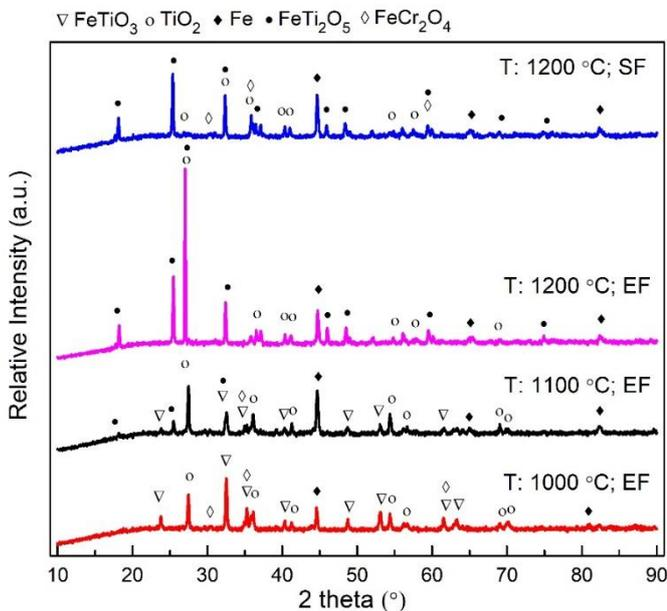
**Figure 1.** XRD analysis results from ilmenite samples carbothermically reduced using an electrically resistant furnace (EF) and a solar simulator furnace (SF).
