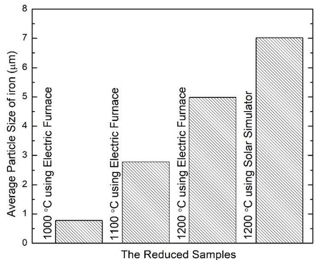
**Figure 2.** The average particle size of metallic iron formed after carbothermic reduction using different heat thermal sources.
