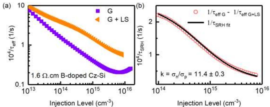
**Figure 2. (a)  $\Delta n$  over  $1/\tau_{\text{eff}}$  of the p-SHJ solar cell before (G) and after (G+LS) LS and (b) injection dependent SRH lifetime curve and model fit.**
