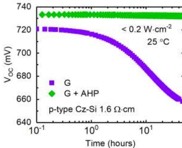
**Figure 1.  $V_{oc}$  as a function of time under illumination for the AHP treated (G+AHP) and non-treated (G) p-SHJ solar cells.**
