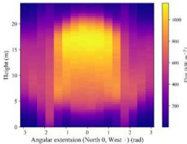
Figure 2: Receiver flux map at design point (Equinox solar noon) showing the prescribed non-uniform aiming on the receiver surface.
