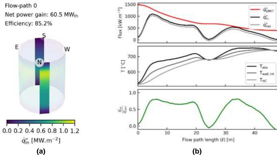
Figure 3: Extract of receiver modelling results: (a) incident flux on a flow-path 0 and (b), from top to bottom, flux, temperature and fraction of allowable flux along flow-path 0 at design point.
