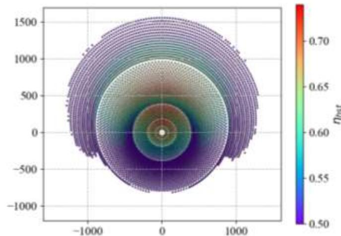
**Figure 1: Heliostat field design obtained from the Single Objective Genetic Algorithm approach.**
