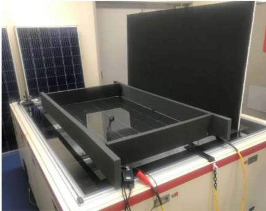
**Figure 2. CSIRO's rear-side light trapping setup**
