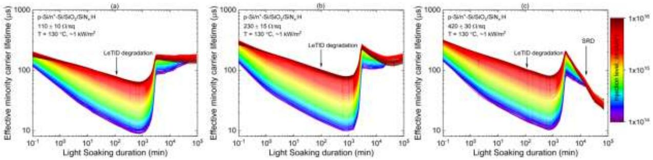
**Figure 3. Injection-dependent  $\tau_{eff}$  as a function of illuminated annealing duration for samples with thermal oxidation and emitter resistivity of (a) 110  $\Omega/sq$ , (b) 230  $\Omega/sq$  and (c) 420  $\Omega/sq$ .**
