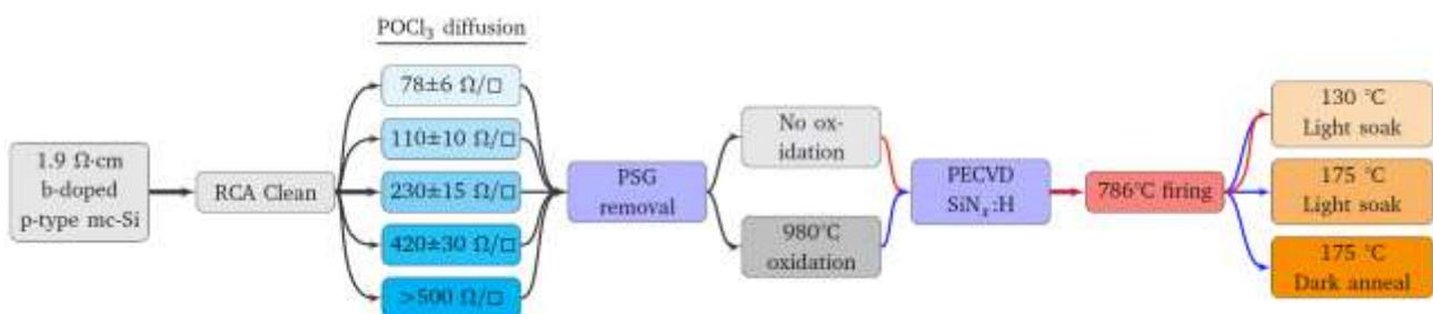
Figure 1. Simplified process flow diagram for the fabrication of test structures
