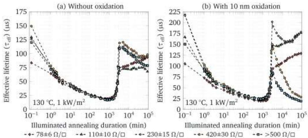
**Figure 2.** Change in  $\tau_{\text{eff}}$  as a function of illuminated annealing duration at 130 °C and  $\sim 1 \text{ kW/m}^2$  for diffused samples (a) with and (b) without oxidation.  $\tau_{\text{eff}}$  is extracted at  $\Delta n = 1 \times 10^{15} / \text{cm}^3$ . The legend refers to  $R_{\text{SH}}$  measured prior to oxidation.
