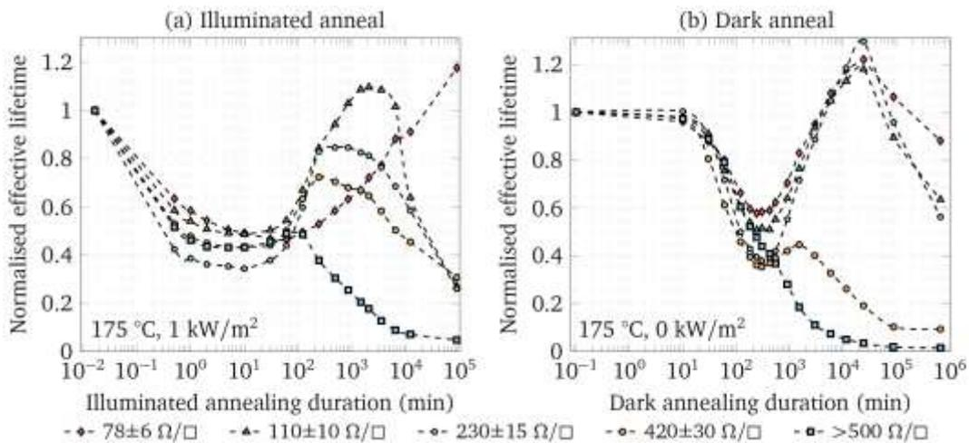
**Figure 4. Change in normalised  $\tau_{eff}$  as a function of (a) illuminated annealing duration at 175 °C and  $\sim 1 \text{ kW/m}^2$  and (b) dark annealing 175 °C.  $\tau_{eff}$  was extracted at an injection level of  $\Delta n = 1 \times 10^{15} / \text{cm}^3$  and normalised to the initial carrier lifetime obtained after firing.**
