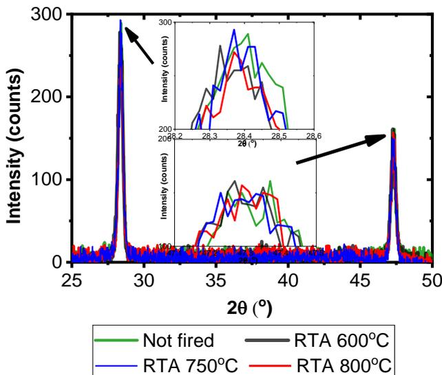
Figure 2. GIXRD results measured on the non-fired samples and the samples fired with RTA at 600°C, 750°C and 800°C.
