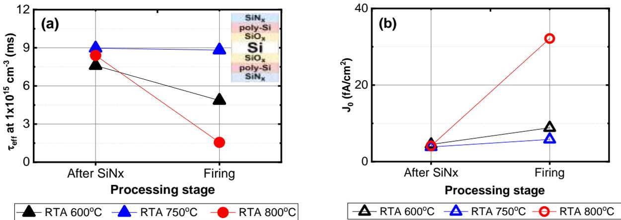
Figure 1.  $\tau_{eff}$  (a) and single-side  $J_0$  (b) values measured before and after RTA treatment at 600°C, 750°C and 800°C.
