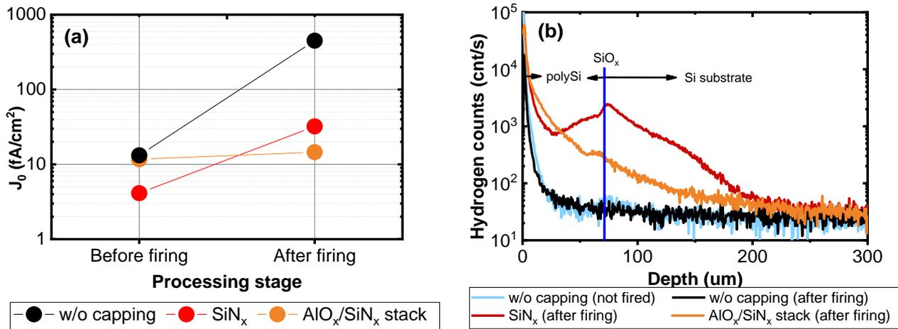
**Figure 3. (a) Evolution of surface passivation quality of samples coated with various dielectric films, and (b) their H signals measured by SIMS.**
