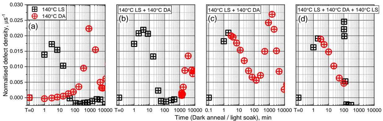
**Figure 1 - NDD of mono-like Si samples upon LS (1 sun) and DA cycles, applied at 140°C.**
