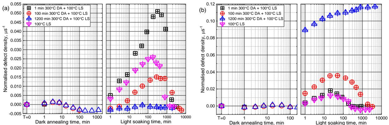
**Figure 2 – NDD of (a) mono-like Si samples and (b) Cz-Si samples during LS under 1 sun illumination at 100°C, after subjecting to an initial DA at 300°C for different durations.**
