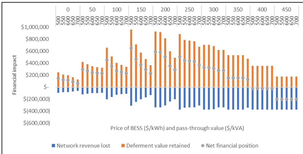
Figure 3. Sum of the financial impacts of the 4 BESS on the network, the network revenue lost is calculated from the difference of applying the network charges to the annual grid import before and after the PV and BESS reductions
