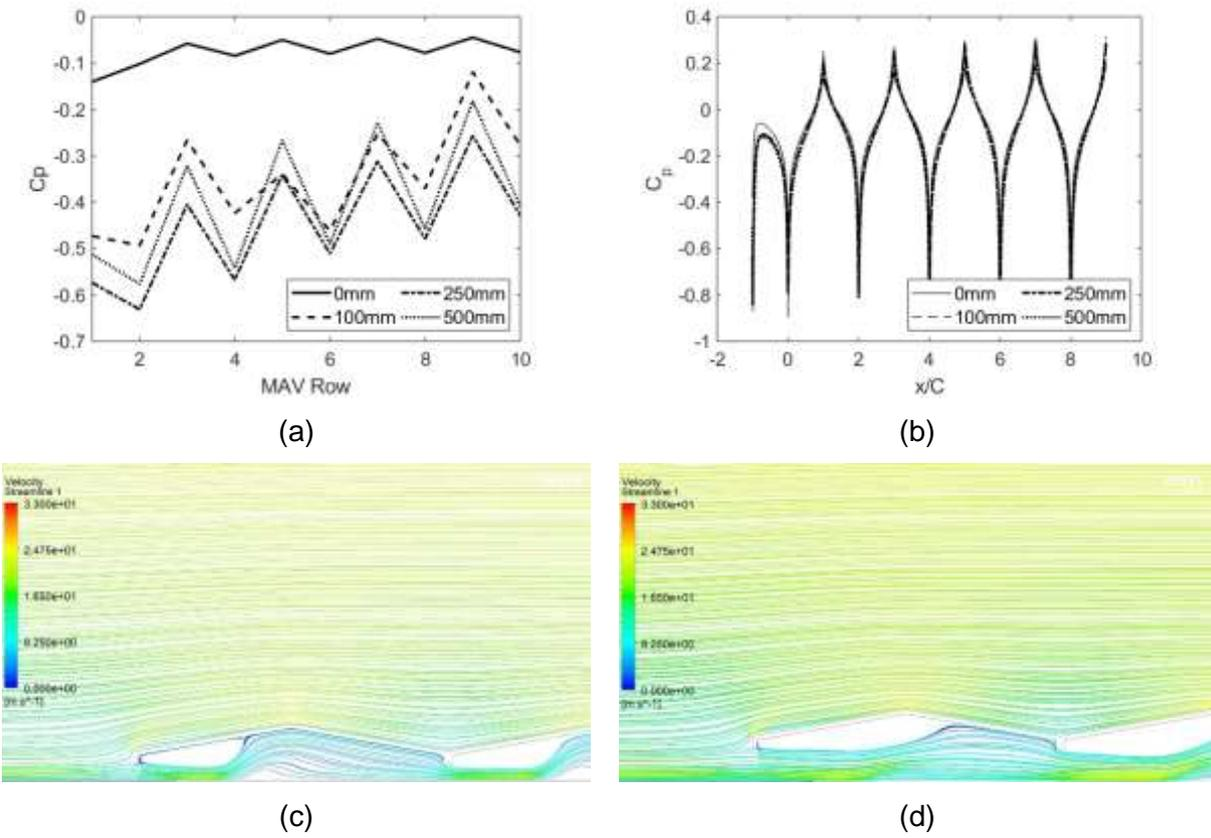
**Figure 2. The effect of ground clearance. (a) shows the average pressure coefficient across each panel; (b) shows the pressure coefficient distribution on the upper surface of the panels; (c) and (d) show the streamlines around the MAV with a 250mm and 500mm ground clearance respectively**
