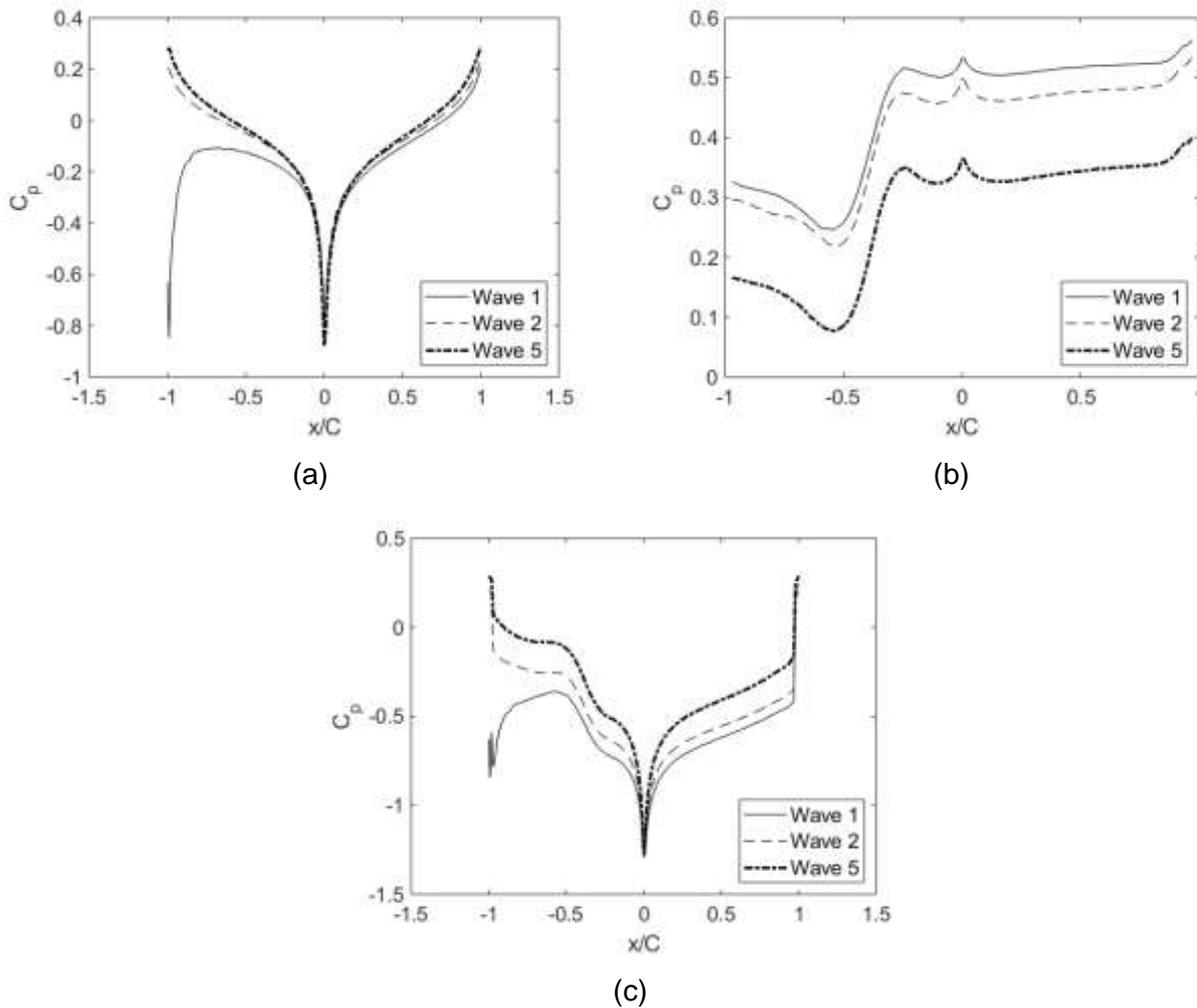
**Figure 3. The effect of row positioning on the pressure coefficient distribution on the (a) upper, (b) lower and (c) net surfaces of the panels with a 250mm ground clearance**
