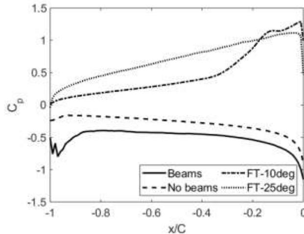
**Figure 4. The pressure coefficient distribution on the first row of east-west arrays with a 500mm ground clearance compared to fixed-tilt arrays at 10° and 25° pitches**
