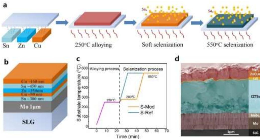
**Fig. 1. Fabrication of CZTSe films and devices.** | **a** Schematics of sputtering, annealing, and two-step selenization processes. **b** Stacking structure of metal precursors. **c** Temperature profiles of the fabrication of reference sample S-Ref and sample S-Mod with modified growth process. **d** Cross-section image of a finished CZTSe device.
