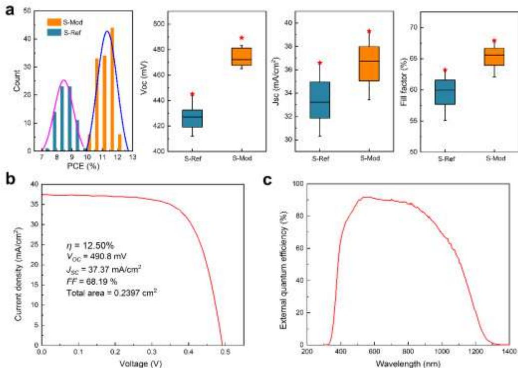
**Fig. 2. Photovoltaic performance.** | **a** Statistical box and histogram plots of device performance parameters of S-Mod and S-Ref. The sample size is 124 cells for S-Mod and 73 cells for S-Ref. All the photovoltaic performance parameters are measured based on total area devices. **b** Certified J-V data and **c**, EQE data of the champion CZTSe solar cell from S-Mod.
