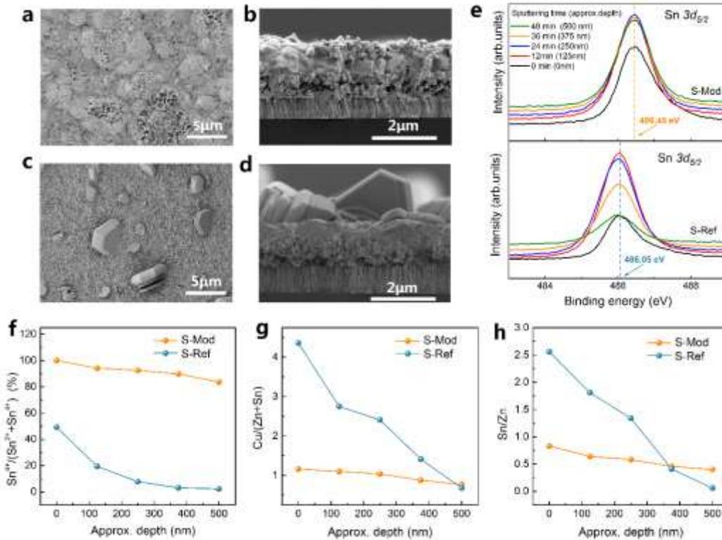
**Fig. 3. Morphologies, oxidation states of Sn, and local chemical compositions of half-selenized samples.** | Surface and cross-section SEM images of **a, b** half-selenized S-Mod and **c, d** half-selenized S-Ref. **e** Sn 3d<sub>5/2</sub> XPS depth profiles of half-selenized S-Mod and half-selenized S-Ref. **f** Depth profile of proportion of Sn<sup>4+</sup> in Sn ions, **g** ratio of Cu/(Zn+Sn), and **h** ratio of Sn/Zn for half-selenized S-Mod and half-selenized S-Ref.
