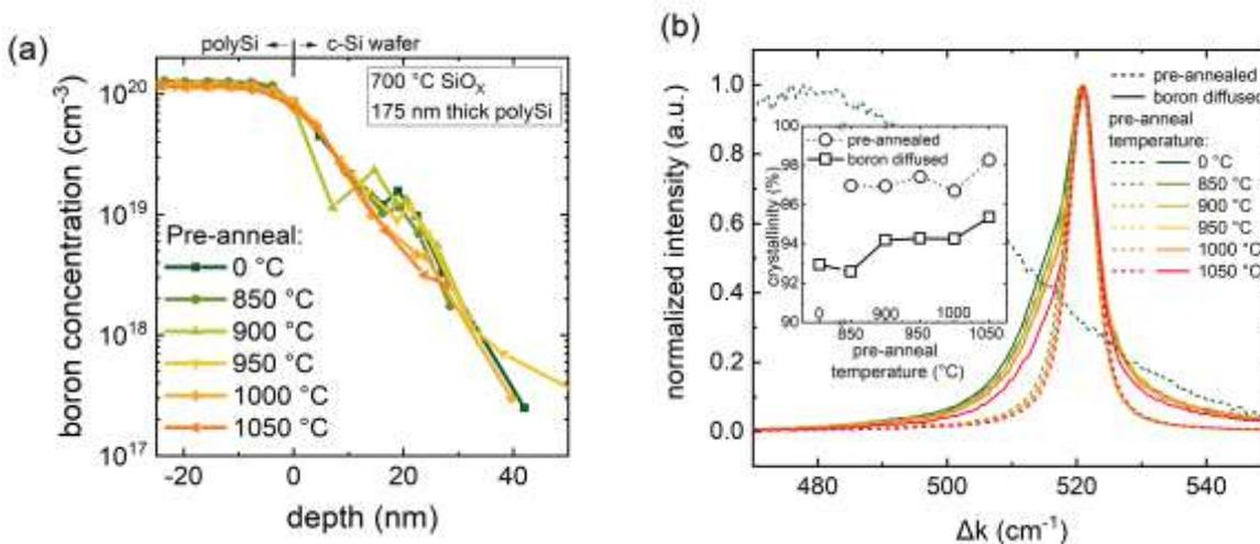
Figure 3: In (a) the active boron doping profiles measured by ECV shown in the region around the interface of polySi/SiO<sub>x</sub>/c-Si. The pre-annealing temperature is varied between 0 °C (no pre-annealing, dark green) and 1050 °C (orange). In (b) normalized Raman spectra before (dotted lines) and after boron diffusion (solid lines) are plotted varying pre-annealing
