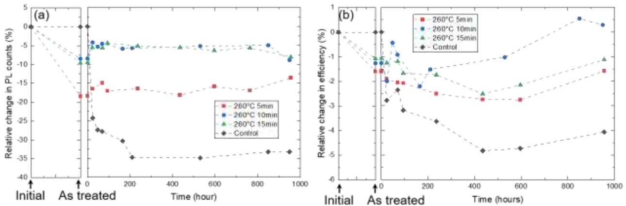
Figure 2. Relative change in (a) PL and (b) efficiency after treatment and during the light soak process for samples bias annealed at 260 °C for 5, 10 and 15 mins and no treatment (control)
