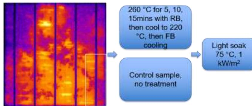
**Figure 1** Diagram of experiment flow for the biased annealing process for treated and control samples
