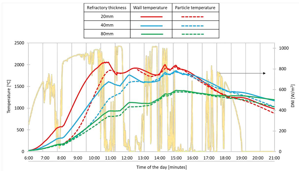
Figure 1. Influence of refractory lining thickness on the transient temperature distributions of the receiver wall and the particles for a fluctuating solar input.
