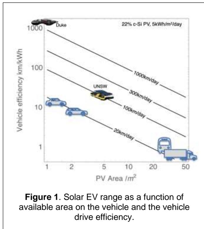
**Figure 1.** Solar EV range as a function of available area on the vehicle and the vehicle drive efficiency.
