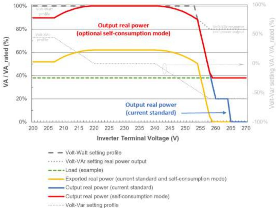
Figure 3. An optional self-consumption mode (Red) for the grid-connected inverter response profile with Volt-Watt and Volt-Var modes of AS 4777.2, allowing the ability for DER owners to self-consume electricity to not be curtailed due to i) high-voltages on the distribution network, or ii) generation shedding mechanisms for security.
