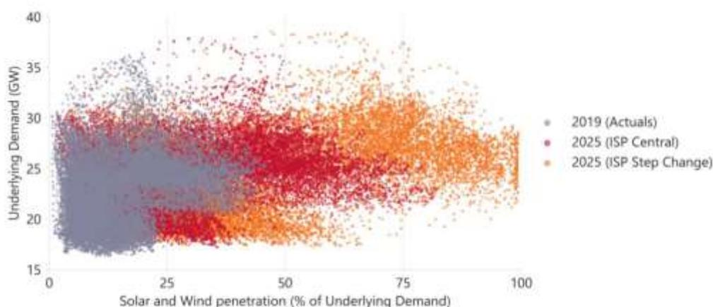
**Figure 1. Australian National Electricity Market half-hourly wind and solar generation divided by the underlying demand, actual and forecast (AEMO Integrated System Plan). Source: Future Energy Systems, AEMO 2020.**
