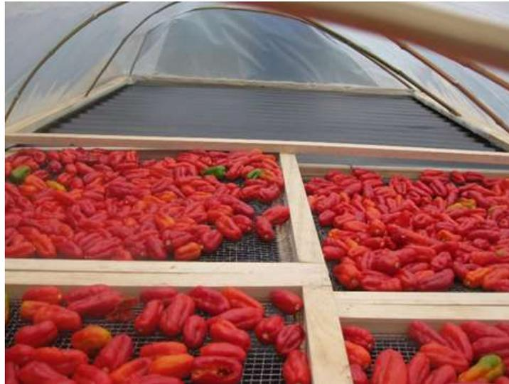
**Figure 3. Preserving chillis in an UNSWERV solar dryer in Port Vila, Vanuatu**
