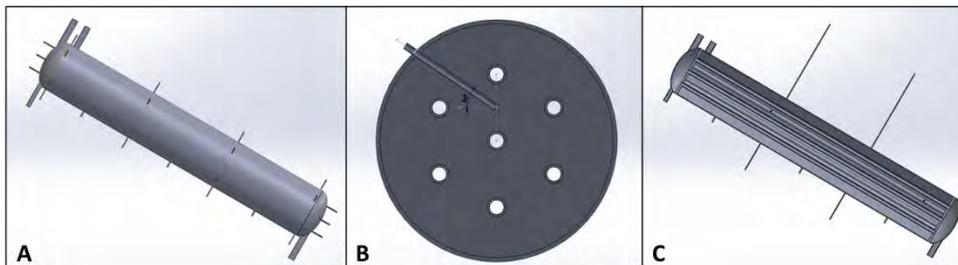
**Figure 1- Design of a High Temperature PCM Storage System for use with Liquid Sodium**
