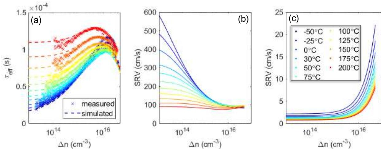
**Figure 2. (a) Measured and simulated  $\tau_{eff}$  for an  $n$ -type Si wafer passivated with 100 nm thick  $\text{SiO}_2$  layer without corona charge. Extracted SRV with (b)  $Q_f = 1 \times 10^{10} \text{ q/cm}^2$  and (c)  $Q_f = 1.6 \times 10^{12} \text{ q/cm}^2$ .**
