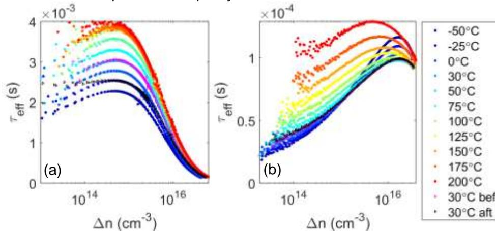
**Figure 1. Temperature and injection dependent  $\tau_{eff}$  for an  $n$ -type Si wafer passivated with 100 nm thick  $\text{SiO}_2$  layer (a) with and (b) without corona charge.**
