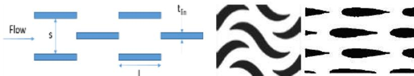
**Figure2- Discontinuous fluid passages between fins; stripe, S shape and airfoil [10]**
