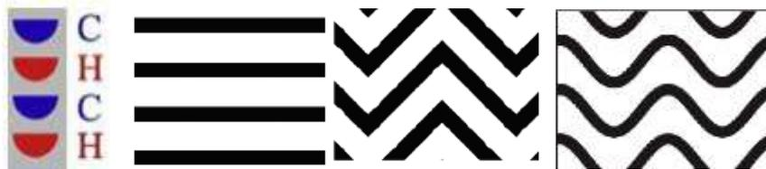
**Figure1- Semicircular cross section in continuous channels; straight, zigzag and wavy**
