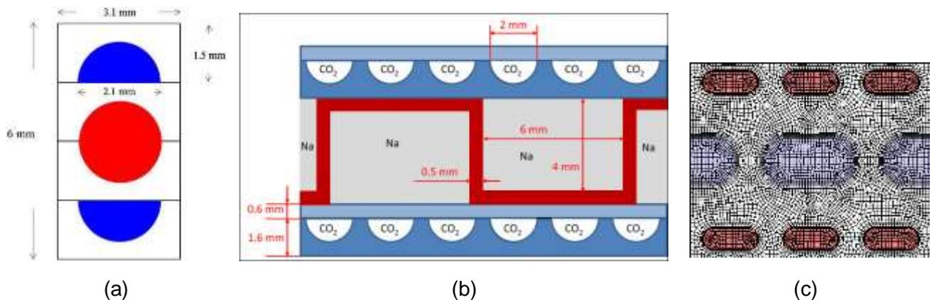
**Figure 3- Circular straight channel for sodium and semicircular zigzag for sCO<sub>2</sub> [11], (b) rectangular straight channels for sodium and semicircular wavy channels for sCO<sub>2</sub> [16], (c) Oval cross section in straight channels for sodium and straight or wavy channels for sCO<sub>2</sub> [this study]**
