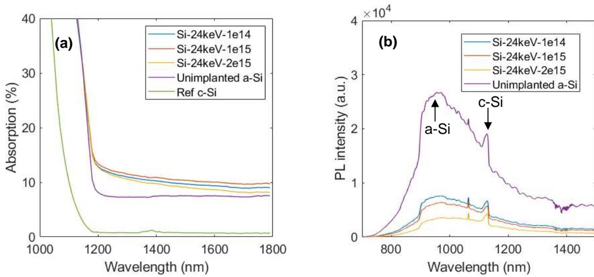
**Figure 2 (a) Sub-bandgap absorption and (b) PL spectra of a-Si containing different doses of implanted Si, measured at 79K.**
