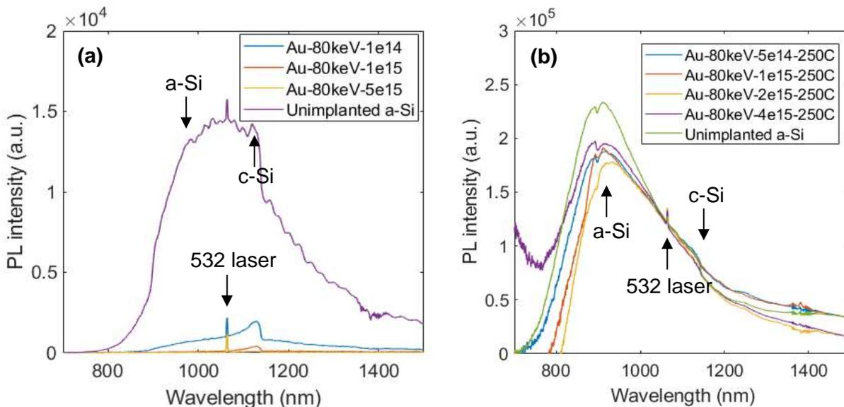
**Figure 3** PL spectrum for a-Si implanted with Au at (a) 300K and (b) 523K at different doses.
