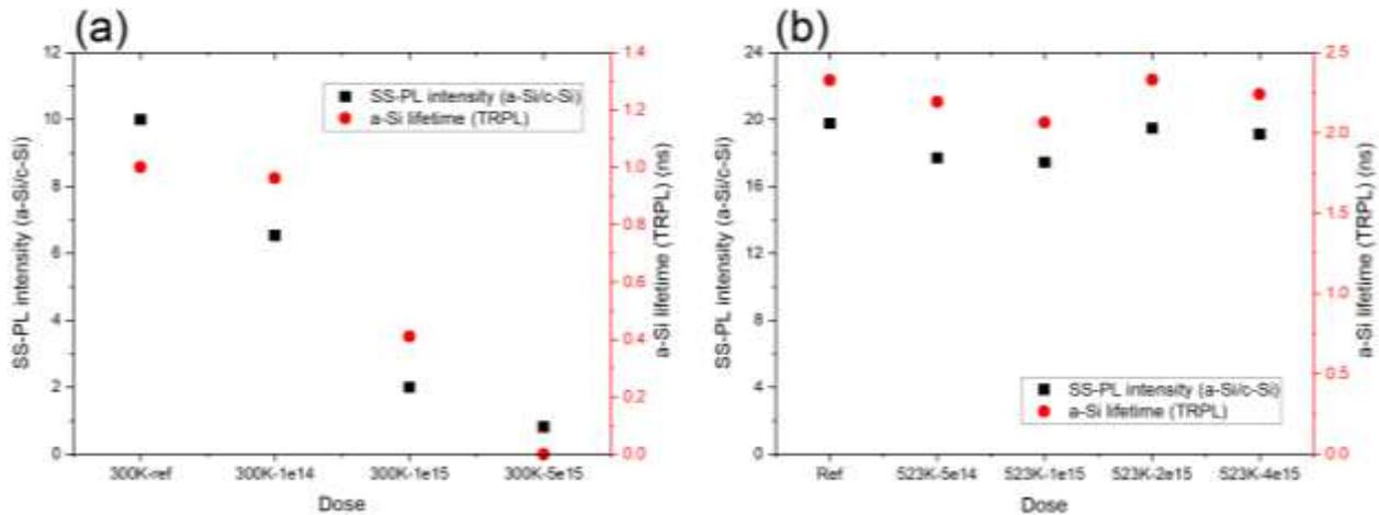
**Figure 4 Normalized steady-state PL intensity from the a-Si layer and a-Si lifetime measured from TRPL for (a) 300K Si-implanted samples and (b) 523K Au-implanted samples. We estimate a 10% error in both the normalized PL signal and a-Si lifetime measurements.**
