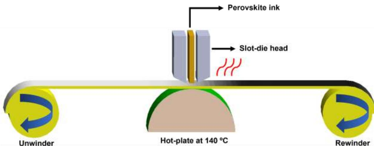
**Figure 1.** Schematic of the employed hot deposition technique for perovskite films fabrication.
