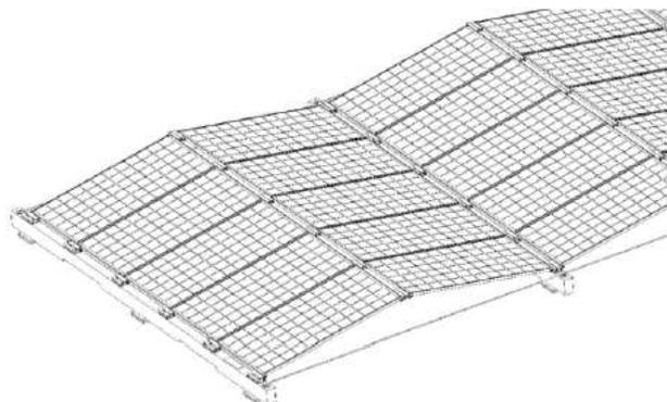
Figure 1: 5B's corner hinge mounted prefabricated array.
