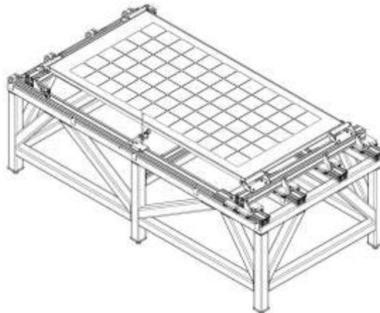
Figure 5: Solid steel test jig designed to enable 5B and standard module mounting configurations
