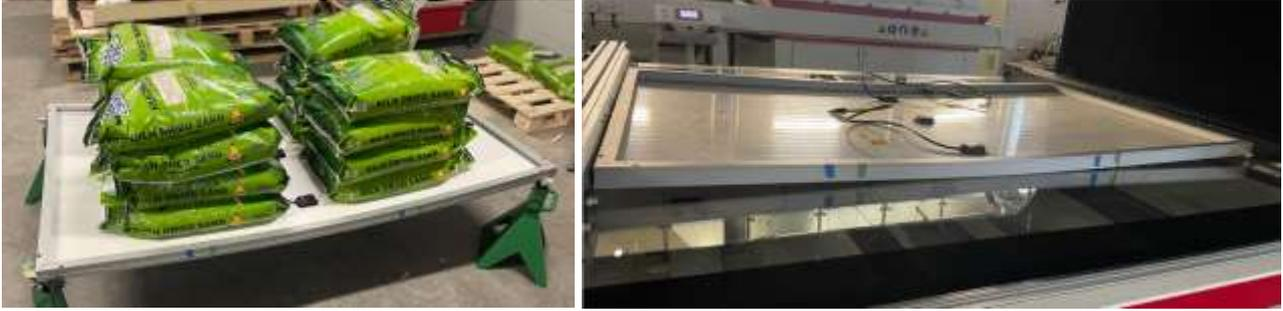
**Figure 2: Standard sized module (a) corner mounted and loaded with 320 kg of sand; (b) plastically deformed (bent) after the load was removed.**
