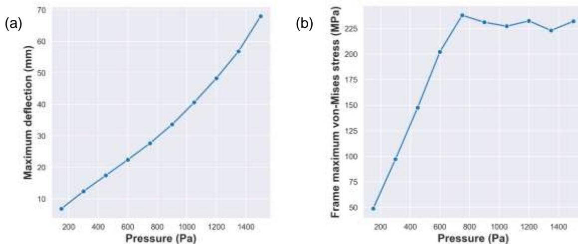
**Figure 7: Simulated utility sized glass-glass module under uplift loading test (a) maximum deflection and (b) maximum von-Mises stress in Al frame as a function of load pressure.**
