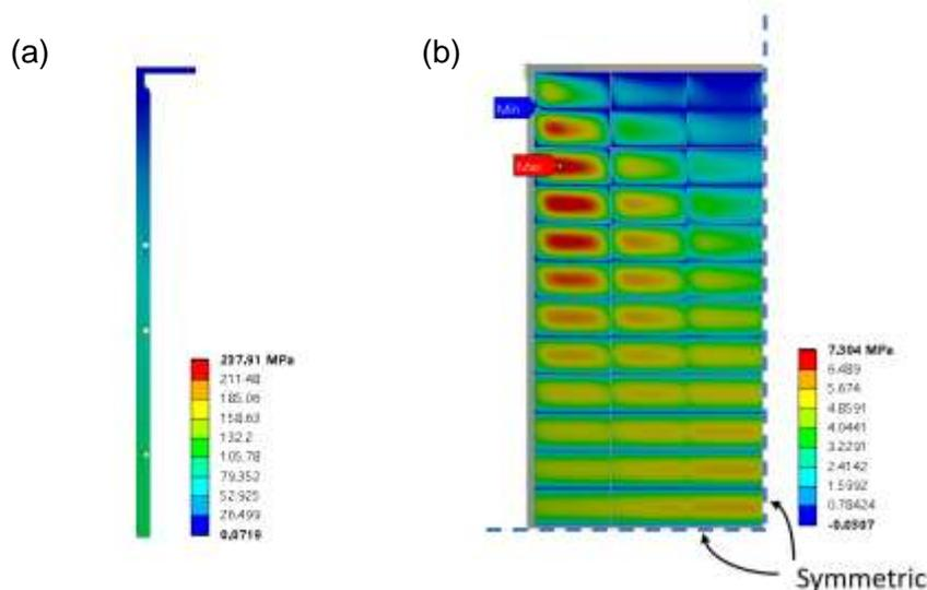
**Figure 8: Simulated 2256 x 1133 mm glass-glass module quarter with 35 mm frame loaded with 750 Pa uplift (a) von-Mises stress in Al frame and (b) tensile stress in Si solar cells.**
