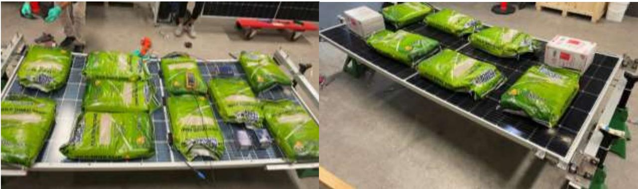
**Figure 3: Utility sized module mounted using 5B corner hinges and loaded (a) from the rear with 202 kg (777 Pa), (b) on the front with 129 kg (494 Pa)**
