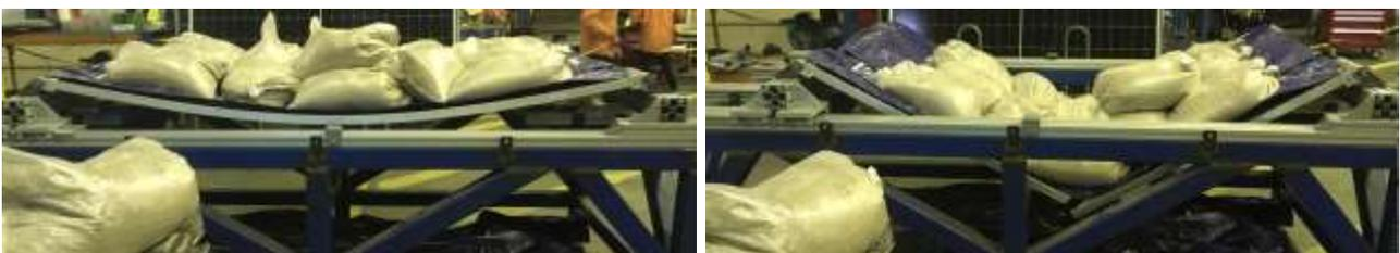
Figure 6: Utility sized module under 335 kg load, (a) before and (b) after failure.
