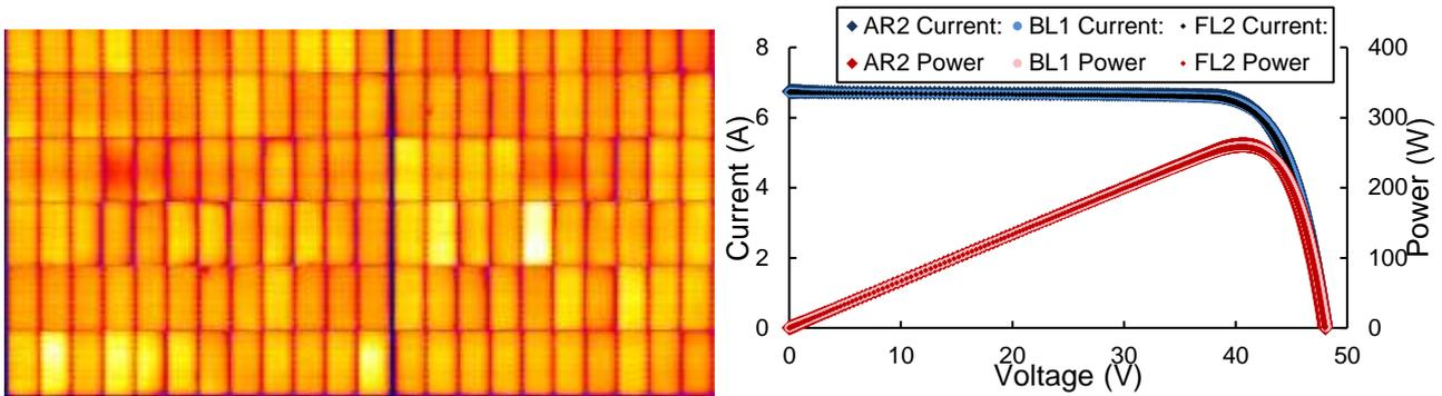
Figure 4: (a) PL image after wind load testing from the front and rear with no microcracks, (b) half-module IV curves as received (AR), after backloading (BL) and front loading (FL)
