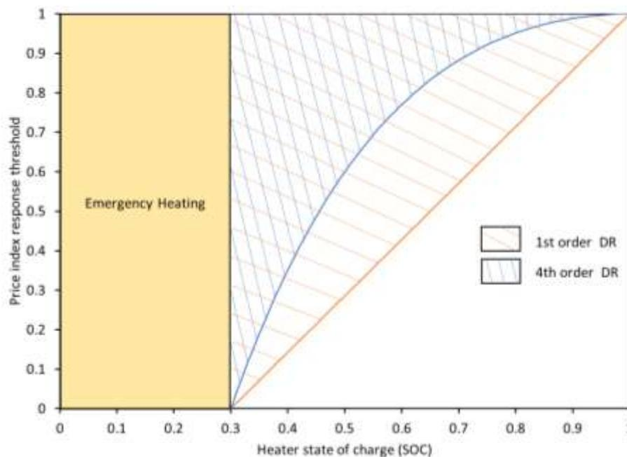
Fig. 2 Dynamic price index response threshold (demand response can operate in hatched area) as a function of heater state of charge.
