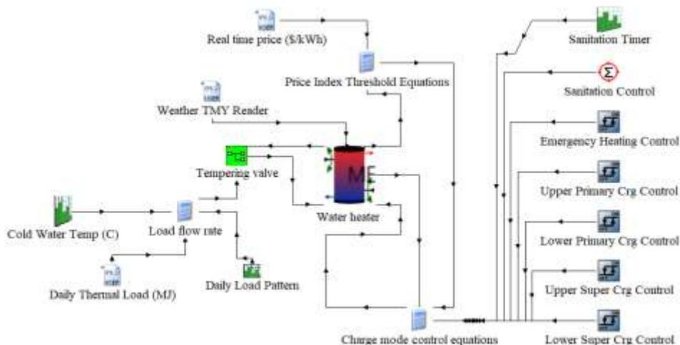
**Fig. 1 Example of TRNSYS schematic of a domestic hot water system.**
