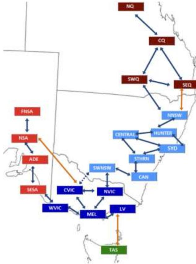
**Figure 1: The NEM transmission model. Blue arrows represent the AC transmission lines, while the orange arrows represent HVDC links.**
