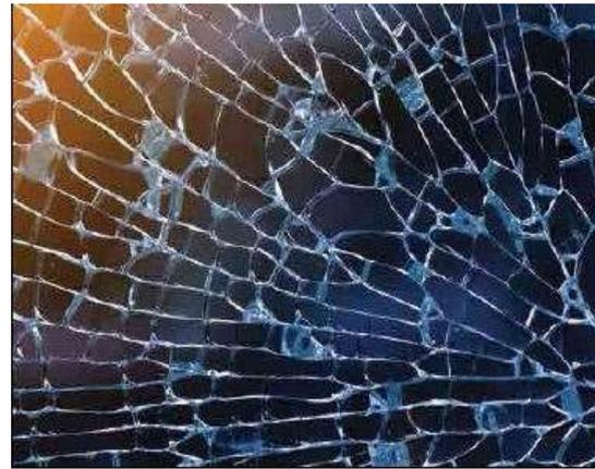
Figure 2: When broken, toughened glass fractures into small granules. [AS 1288]
