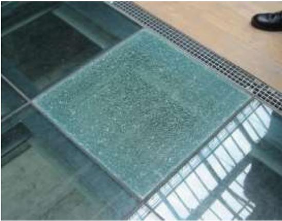
Figure 1: A floor element in laminated glass with the upper ply<sup>[5]</sup> .
