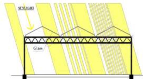
Figure 3: Prototype for Glasshouse (Front View) Yellow shaded portions<sup>[7]</sup>: - Direct solar radiation at Mediterranean latitudes. [21 June, 12:00 pm]
