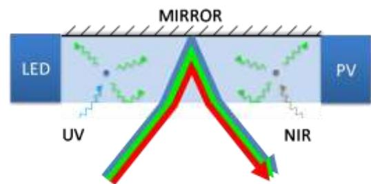
**Figure 2. Luminiscent concentrator and light glow system applied as a secondary reflector for a building integrated heliostat system. The device absorbs UV and Infrared light while reflecting visible light.**
