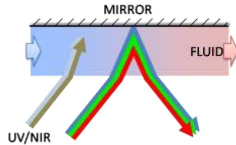
**Figure 4. A fluid contained within a cavity on the front side of a mirror is used for thermal energy extraction. Addition of particles to the fluid can make the device act as a switchable diffuser.**
