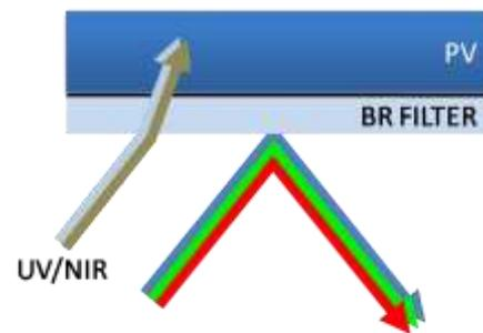
**Figure 3. Band reject filter designed to reflect visible radiation (looks like a mirror), while also generating electricity with a PV cell.**
