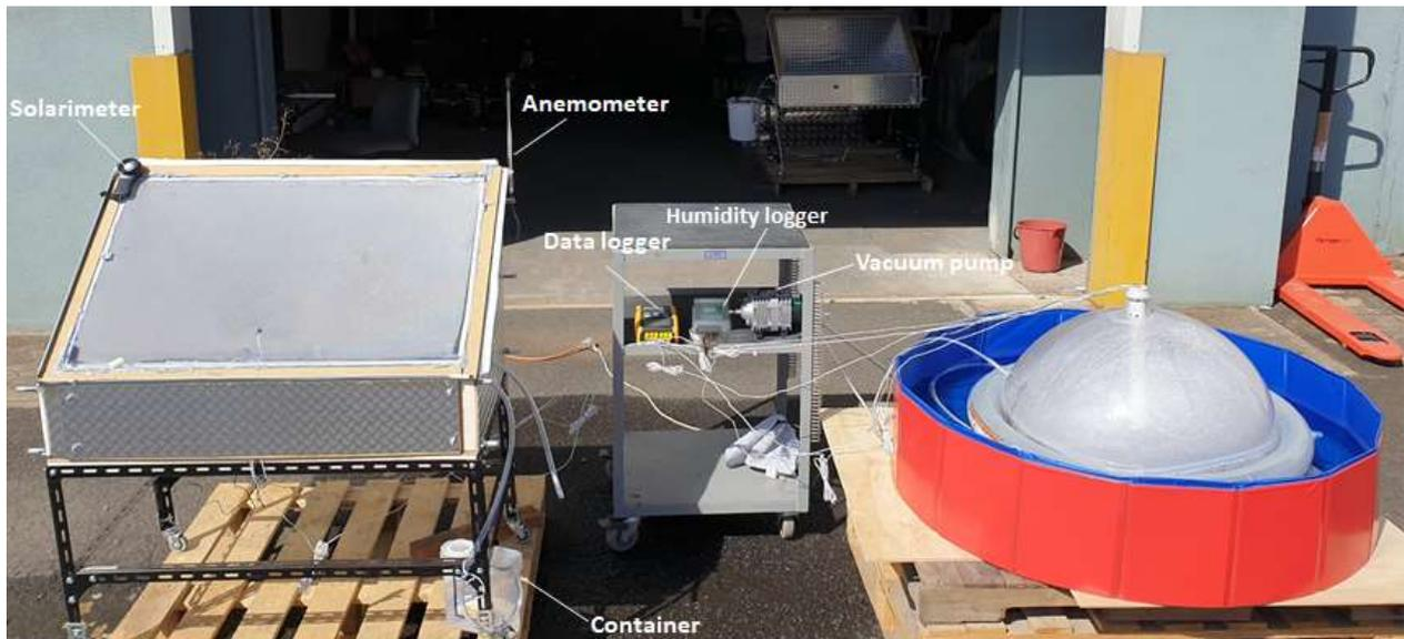
**Figure 4. Photograph of the outdoor experiments of FHSD next to CPSS.**
