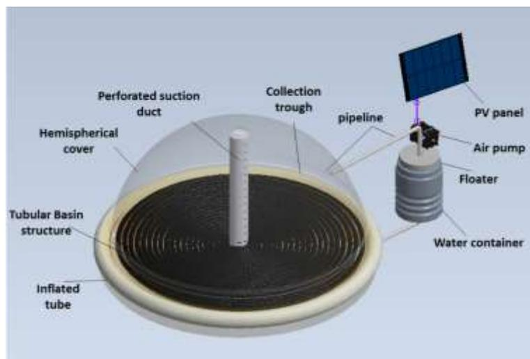
**Figure 2. Schematic of the floating hemispherical Solar Still.**
