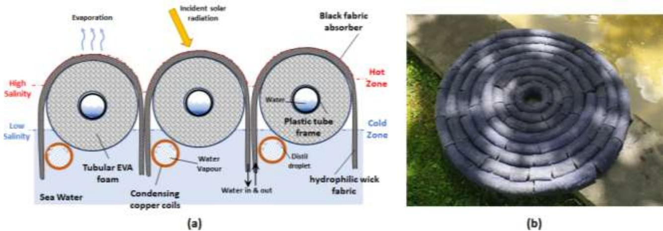
**Figure 1. Schematic and photo of the floating multi-layer basin structure**
