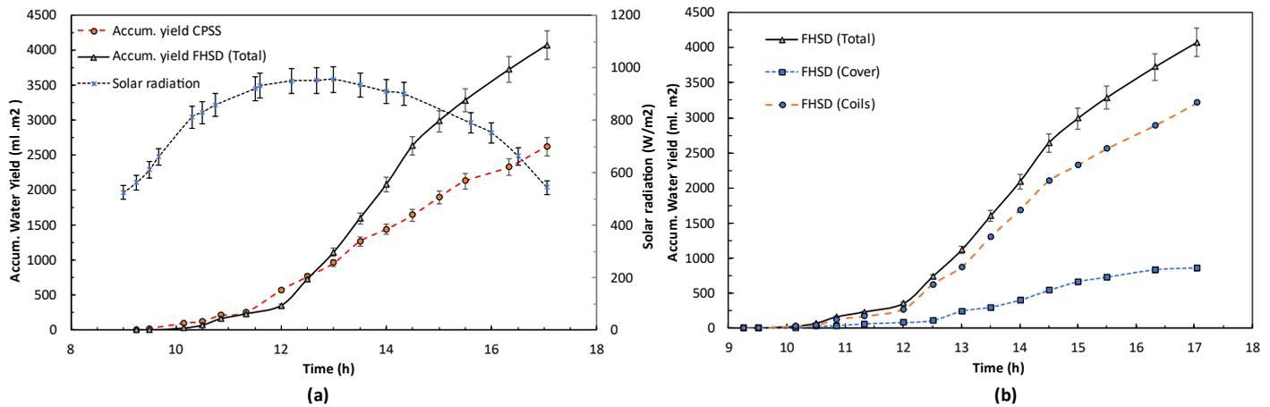
**Figure 3. (a) Accumulated water yield for FHSD and CPSS setups; (b) Deviations of accumulated water yield distilled on the cover and the coils of FHSD.**
