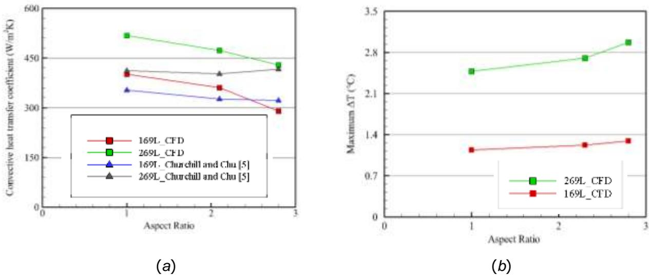
**Figure 3.** (a) Comparison of sidewall convective heat transfer coefficient predicted by CFD model and vertical flat plate correlation of Churchill Chu (Churchill and Chu, 1975) and (b) Maximum temperature difference of water within the tank reflecting the degree of thermal stratification
