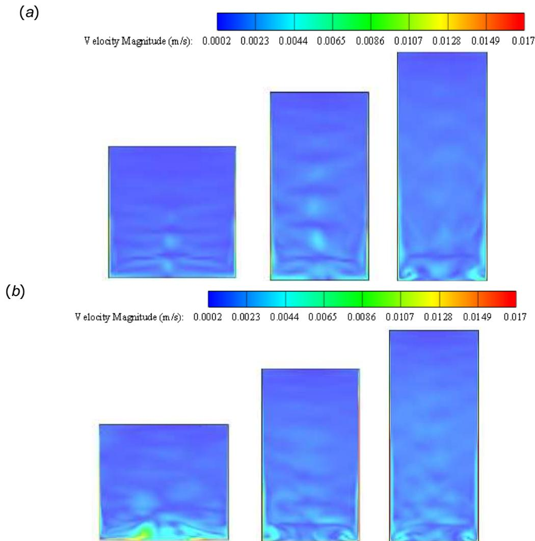
**Figure 4.** Velocity contours of tank models with various aspect ratios with tank volumes of (a) 169L and (b) 269L
