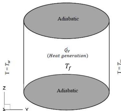
**Figure 1.** Schematic of the computational boundary conditions
