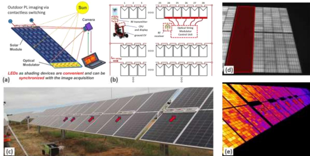
**Figure 1.** (a) Outdoor PL imaging of single module via contactless switching; (b) principle of outdoor PL imaging technique based on PV string modulation; (c) optical modulators (red arrows) on PV module string; (d) PL image of a full module with faulty bypass diode; and (e) outdoor PL image of several modules in a PV string.
