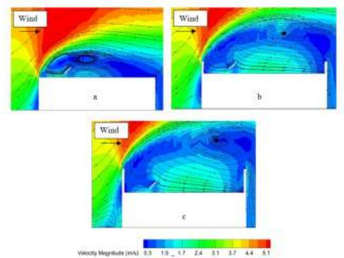
**Figure 3: Streamwise velocity path lines and contours show the collector's main flow features at varying parapet heights.**
