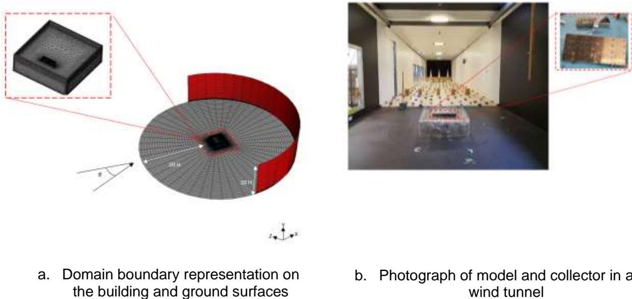
**Figure 1. Numerical and experimental set-up**
