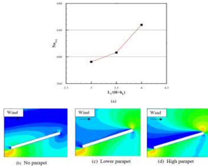
**Figure 4: (a) Average Nusselt number at varying parapet height ( $\theta=0^\circ$ ,  $\beta= 20^\circ$ ,  $V=5\text{m/s}$ ; collector located 25 per cent of roof cavity to incoming wind);  $L_r$  is the length of the roof cavity,  $H$  the height of the building and  $h$  height of the parapet  $h_p$ . (b-d) Velocity contours for local velocity around the collector.**
