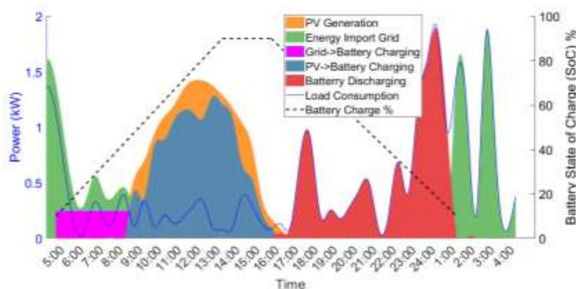
**Figure 2: Battery arbitrage scheme operation in a 3.7 kWp PV system.**
