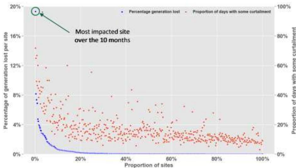
**Figure 1 Distribution of D-PV tripping curtailment: percentage of total generation being curtailed and proportion of days with curtailment occurring for 500 D-PV sites**
