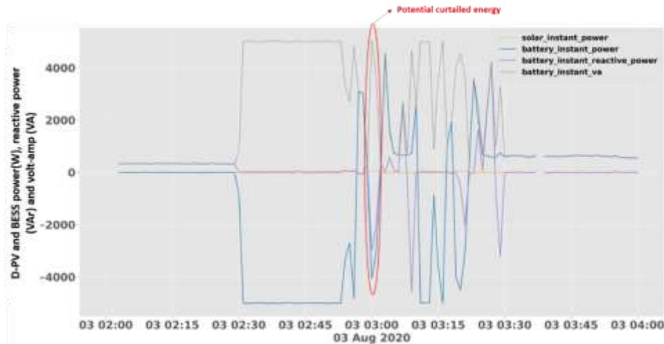
Figure 4 Example daily operation from a sample BESS where V-VAr curtailment can be observed
