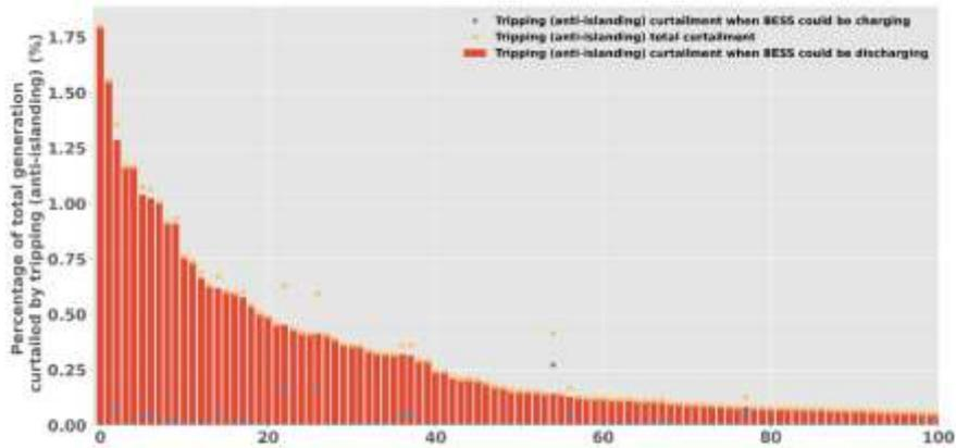
Figure 2 Percentage of total generation curtailed by tripping (anti-islanding) for 100 BESS sites with highest tripping curtailment
