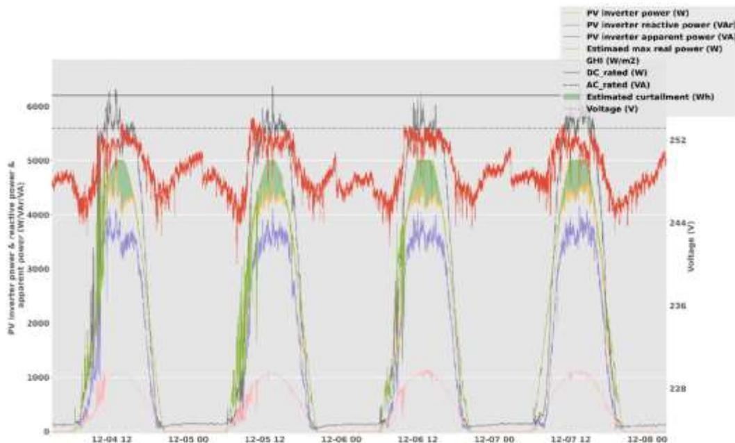
Figure 3 Example operation from a sample D-PV inverter where energy curtailed by V-VAr is highlighted by the green shaded area
