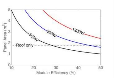
**Figure 2** : PV capacity as a function of area and efficiency. A typical EV has less than  $2m^2$  of available area on the roof. Figure reproduced from [5]
