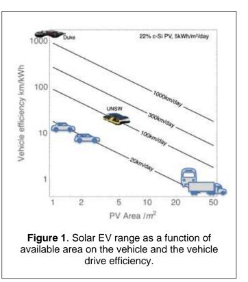
prototype solar Prius is already operating at 17km/day drive and the UNSW 'cruiser class' solar car racer built by the SunSwift student team achieves 34km/kWh, delivering a solar range over 100km/day. To illustrate the dramatic potential for improved vehicle efficiency, it is worth noting that the world record for vehicle efficiency was set by Duke University, achieving 1283km/kWh [6].
