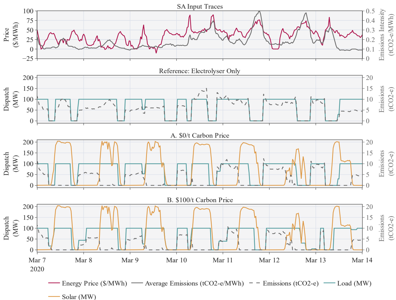
Figure 1 Impact of shadow carbon pricing on electrolyser operation.
