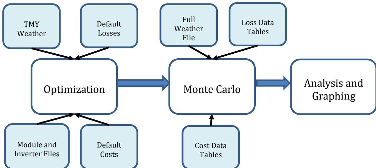
Figure 1: Block Diagram of Simulation Processes
