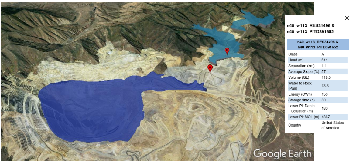
Figure 1: Potential 150 GWh PHES using Bingham Canyon mine. Upper reservoirs (light blue), lower reservoir (dark blue), tunnels (white), dam walls (grey), cost classes (red pins), and an infographic box are depicted.
