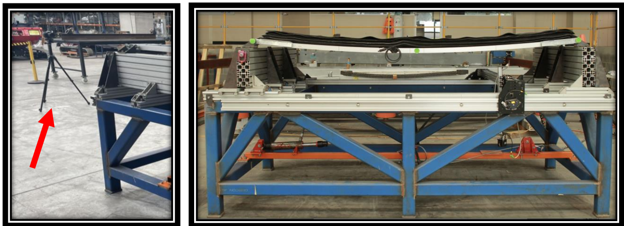
Figure 3: (a) The tripod mounted camera (b) an example image from the camera showing the setup and frame deflected under load.
